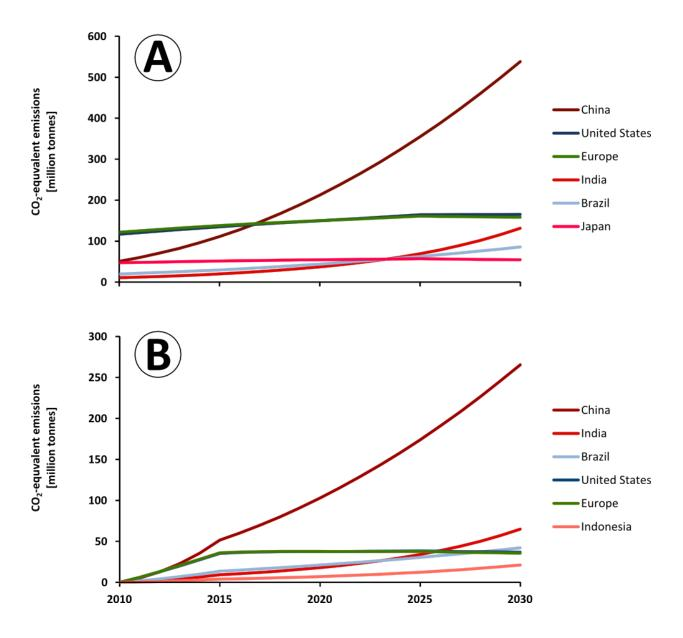
Figure 30: Projected total (direct and indirect) emissions from AC equipped cars for the top-6 countries as calculated by a vintage bottom-up stock model (A). Key determining factors are stock and sales figures. The upper graph (A) shows the BAU scenario, while the bottom graph (B) shows the mitigation potential.
