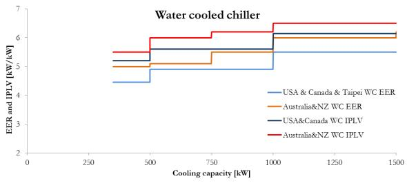
Figure 32: MEPS EER and IPLV requirements for AirC (A) and WC (B) chillers.
