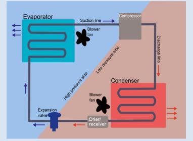
Figure 6: The refrigeration cycle. The refrigerant is under high pressure on the red side and heat is rejected. There is low pressure on the blue side and heat is absorbed
