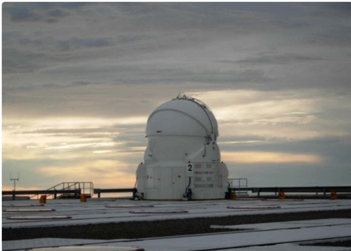
Schmitt, G. 2007. One of the 1.8m diameter auxiliary telescopes, mobile on tracks, working in synchronization with the large telescopes. [Photograph]. Paranal, Chile.
