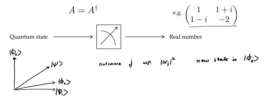
• An observable A for a k-level system is an operator: a kxk Hermitian matrix.
