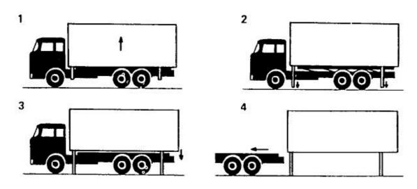
Figure 5: Unloading principle of the swap body. (source: Jensen, 1985, with kind permission)
