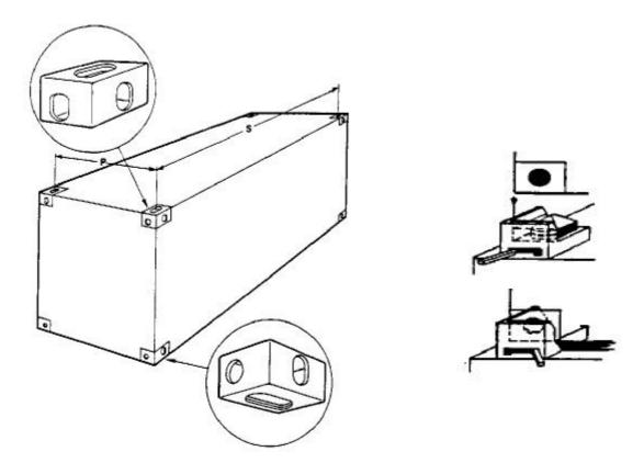
Figure 4: Corner fittings of the ISO container and the twistlock mechanism (sources: ISO/R 668 corner fittings, and SIS standardisation archive (1966), with kind permission from the NNI, Delft, and the SIS, Stockholm).
